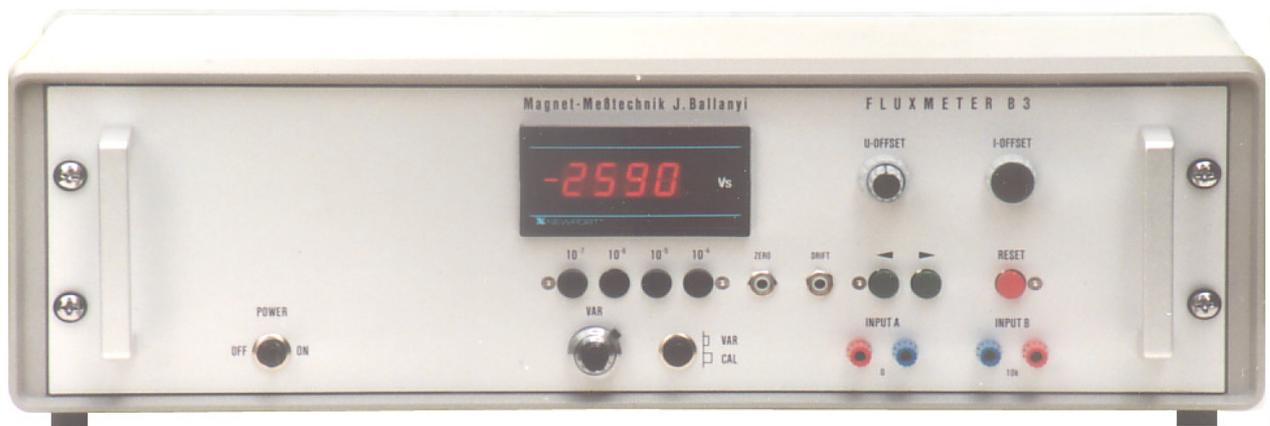
The Fluxmeter B3 is an electronically integrating measuring bench unit with digital display, very low drift and high sensitivity.
