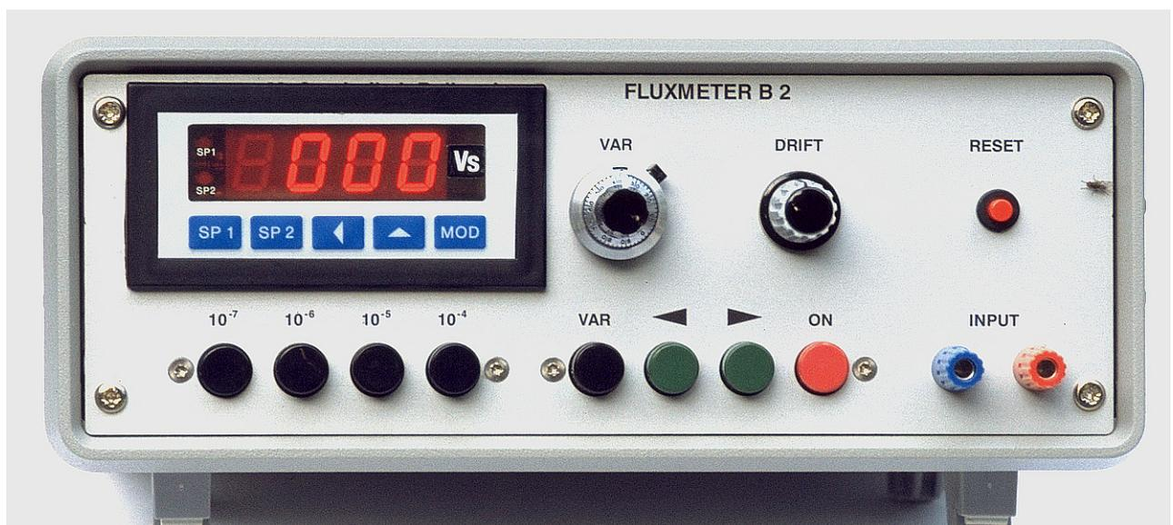
The Fluxmeter B2 is an electronically integrating digital display instrument featuring high sensitivity and low drift. Its versatility permits utilisation in the laboratory as well as in production.
