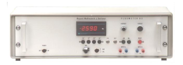
The Fluxmeter B3 is an electronically integrating measuring bench unit with digital display, very low drift and high sensitivity.
